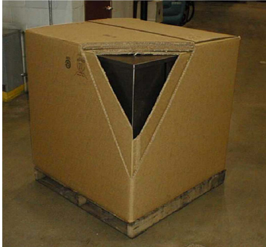
Metal-lined double tri-wall corrugated carton on a wood pallet
